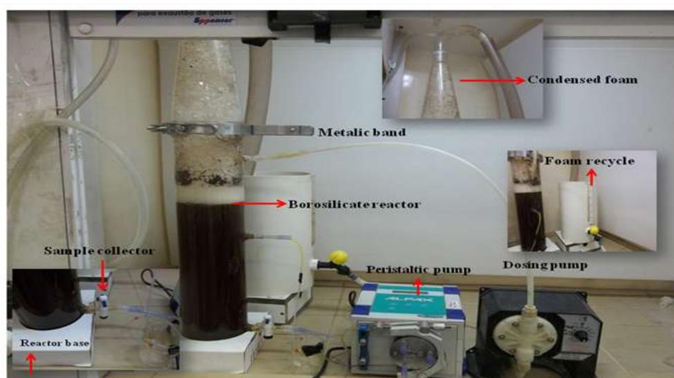
Figure 1— Fenton oxidative process reactor
